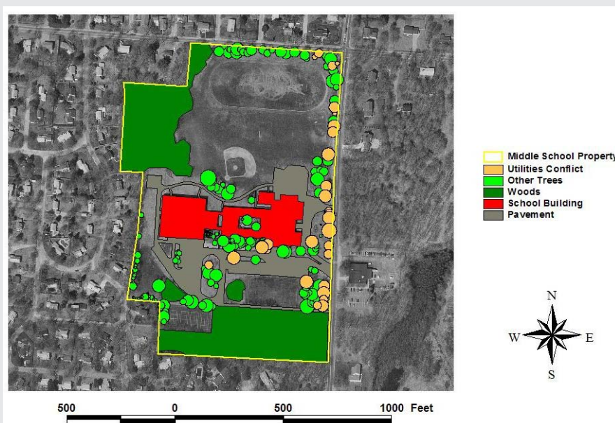
FIGURE 8.5 Trees conflicting with utility lines.
