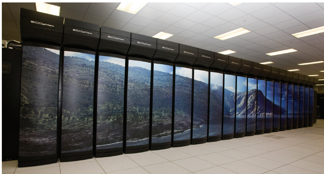
FIGURE 1.5 Global climate models are run on supercomputers, like the NOAA climate research supercomputer Gaea at Oak Ridge National Laboratory in Tennessee (pictured). It has a peak speed of 1.1 petaflops (more than 1,000 trillion calculations per second). SOURCE: ORNL photos/Jay Nave ( http://blogs.knoxnews.com/munger/2011/12/noaas-petascale-computer-for-c.html ).
