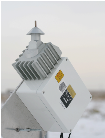
Figure 2 – ASOS B.F. Goodrich Ice Detector Sensor.
