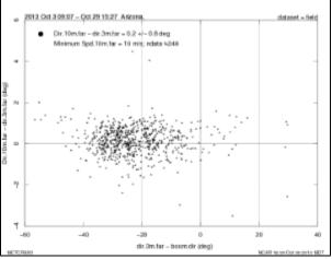
10/8, At FLR, the 2D sonic was pointed nominally north, but must be off by 180 degrees. The median value of Dir.10m + 180 - dir.3m = 6.6 +/- 5 deg. Thus need to add 180 - 6.6 = 173.4 deg to 2D wind direction data.
