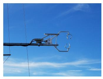
Reshot boom angles of sonics at 10 m and 3 m. The 2D sonic at 10 m had an azimuth of 319 deg. The 3D sonic azimuth was 227 deg.
