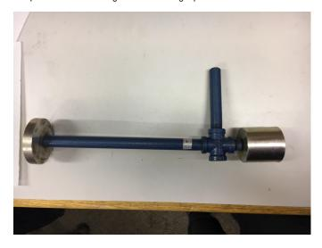
I had left the rod + weight on while using the sledge on it because I hadn't wanted to bang up the top of the pipe too much, but apparently this was worse. I think either the rod is slightly bent or the top of the pipe got beaten out of shape enough that the rod no longer comes out. Liz and I might spend more time trying to get it unstuck tomorrow.
