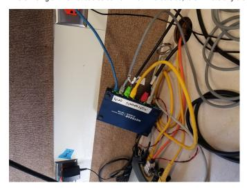
Ethernet switch on the countertop after re-plugging connections to remove lateral forces. The black Ethernet cables with the red plug is an outdoor cable (used for the DSM, I believe) and was pulling sideways on the switch and may have been causing connectivity issues. I may remount the switch on the wall above the hole in the countertop to alleviate the issue and get the switch back off the countertop surface.
