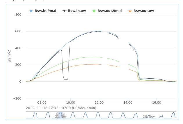
Second, today I see Rsw.out.9m higher than the incomings at 15:00. Usually, I'd blame this on snow covering the incoming sensors, but Rsw.in.9m is within a CVF4 housing that <should> be keeping it clean. Also, Rsw.in from the NR01 tracks Rsw.in.9m quite well, even though it has no housing and a different construction. Thus, I'm inclined to think that this is a real reflection somehow.
